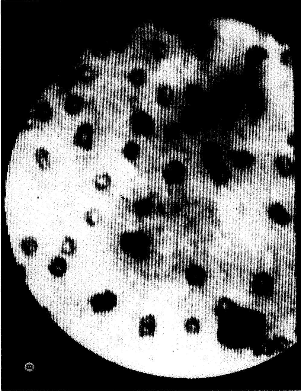
FIG. 1. Fe/TiO 2 during reduction at 770 K. (A) Upon commencement of reduction; (B) same field after 1 h reduction.
